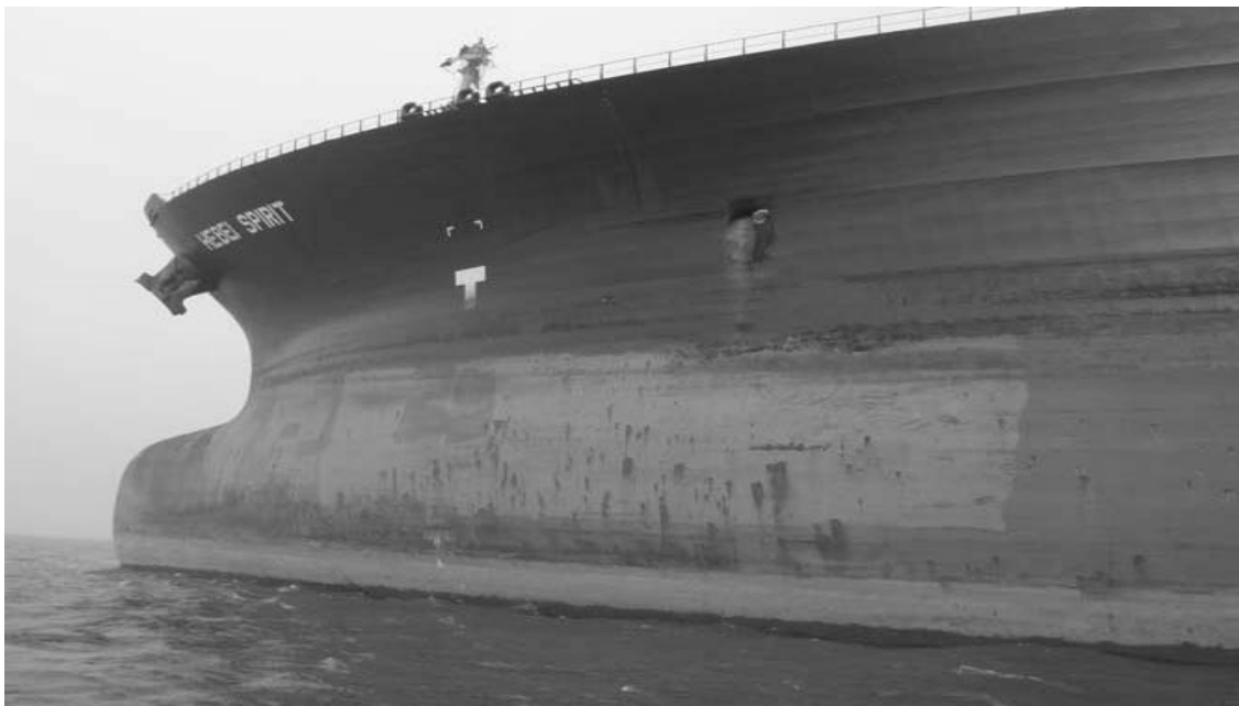
Fig. 4 Damaged No. 1 port cargo oil tank
