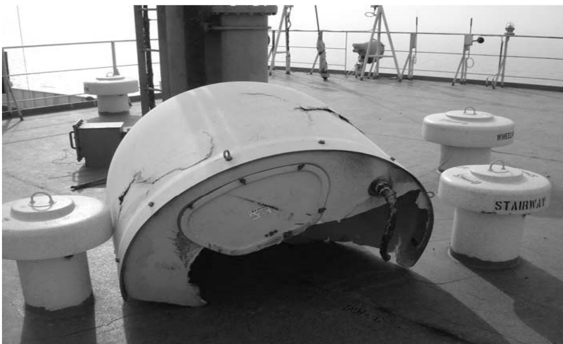
Fig. 5 Damaged satellite communication dome at the main mast
