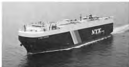
Fig. 9 PCTC installed with 8UEC60LSII-Eco
