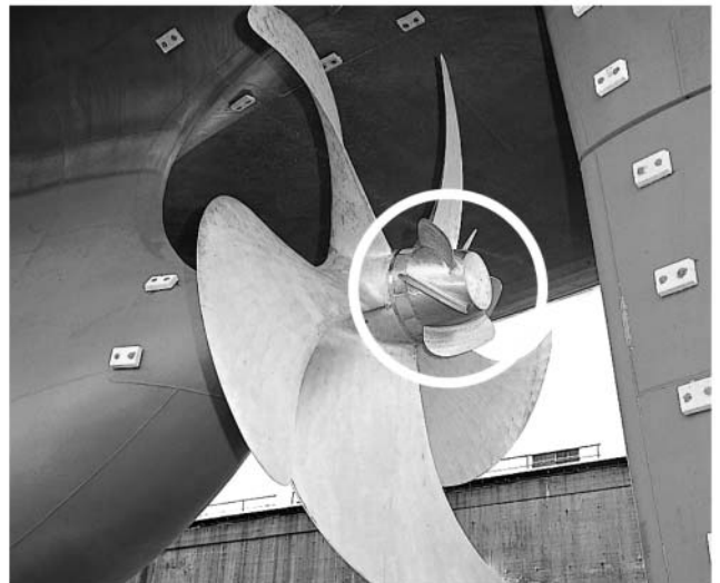
PBCF bolster the propeller's propulsion efficiency
