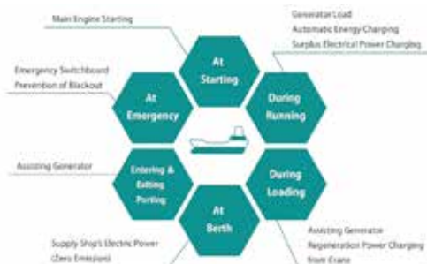
Fig.1 Applications of Li-ion Batteries on Ships
