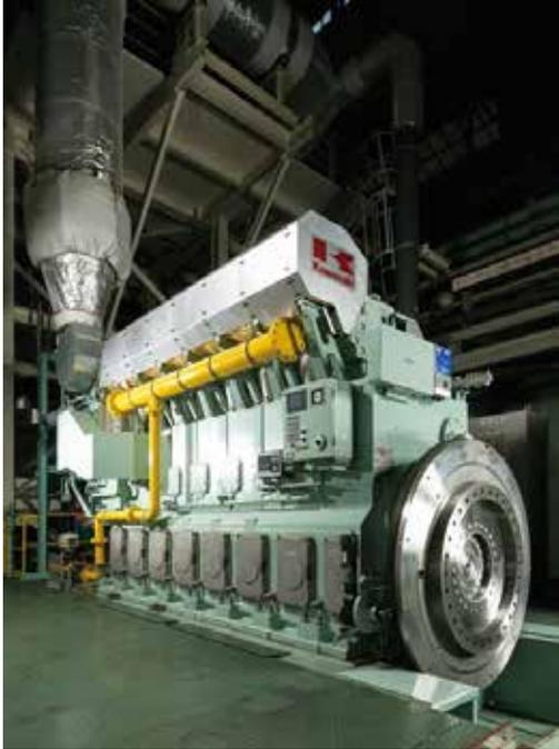
In April 2014, Kawasaki Heavy Industries, Ltd. obtained the type approval certificate from DNV-GL for Green Gas Engine L30KG — the main engine for large vessels fueled solely by gas with an output capacity of over 2 MW.
