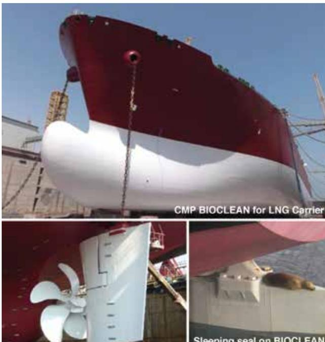
Foul-release coating (FRC) is one of the environmental choices of antifouling and has proven application records since 2003.
