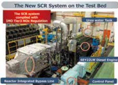
YANMAR developed SCR System that meets to IMO Tier3 regulations.
