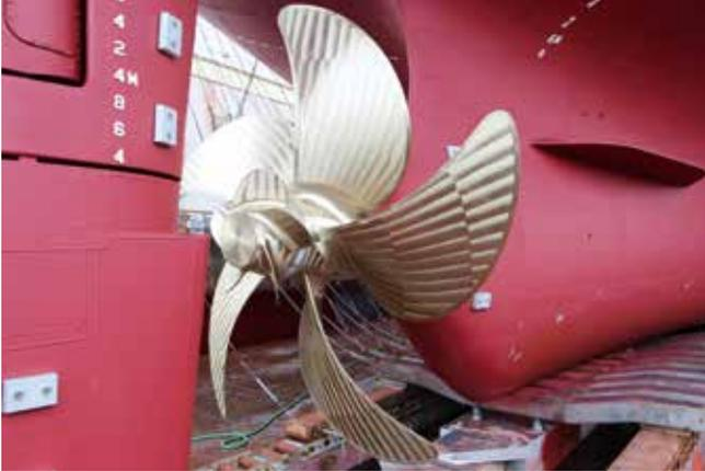
PBCF is the pioneer and the best seller in an energy-saving device installed on a propeller to improve propulsive efficiency by eliminating hub-vortex and by reducing torque loss. In consequence, vessel fuel consumption will be reduced by up to 5%. Mitsui O.S.K. Lines (MOL) originally developed PBCF in 1987, and advanced PBCF was released in 2017. The total number of installation is now over 3,400 vessels all over the world.
