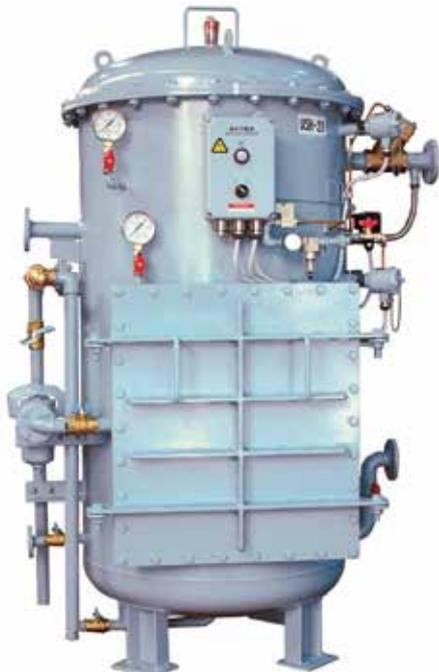
TAIKO's USH series of marine bilge separators was developed by combining the technology of our three previous bilge separators when MEPC.107 (49) took effect., The USH series of new and powerful bilge separators is equipped with a high-performance, long-life coalescer capable of dealing not only with high-density and viscosity oil, but also emulsions that previous coalescers could not deal with.
