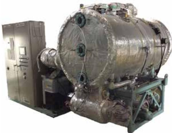
The VVC distiller system has four main components; a horizontal-tube, thin-film evaporator; a rotary blower and a back-up heater. Vacuum in the unit is maintained by a small vacuum pump.
