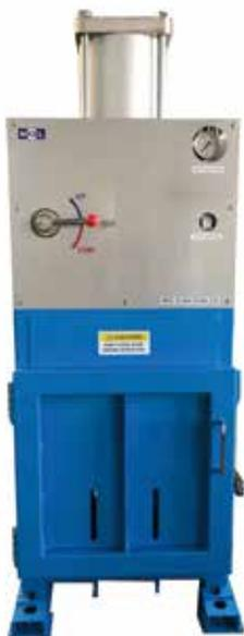
MOL Techno-Trade, Ltd. newly developed air actuate Garbage Compactor AGC-III which can compress various waste materials such as plastic film, bottle and beverage cans by using compression air onboard. Simple design with easy and safe operation will be much effective for organizing waste materials. AGC-III can also reduce the waste disposal cost.
