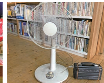
A portable battery of 250W, which can run a fan for 6 hours.
