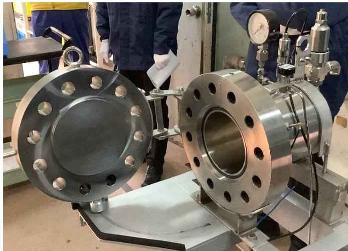
4. Japan performed 12 and 19 tests for the low- and high-water content ANEs (see Figures V and VI). In the initial stage of the tests, the initial pressure was set with reference to the MBP described in the MTC. The initial pressure of the vessel was increased or decreased to properly evaluate MBP according to GO/NOGO results.
