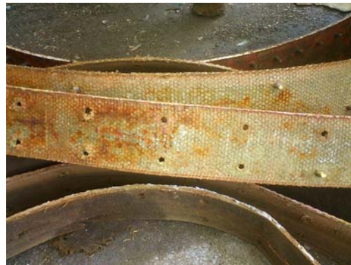
(Brake lining for windlass)
