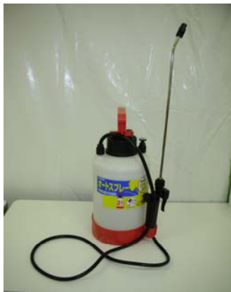
Photo 5 Apparatus used for spraying water (Auto spray ε-value AS-2500N)
