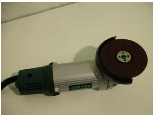
Photo 7 Process 2 Disc sander (Hitachi PDA-100F)
