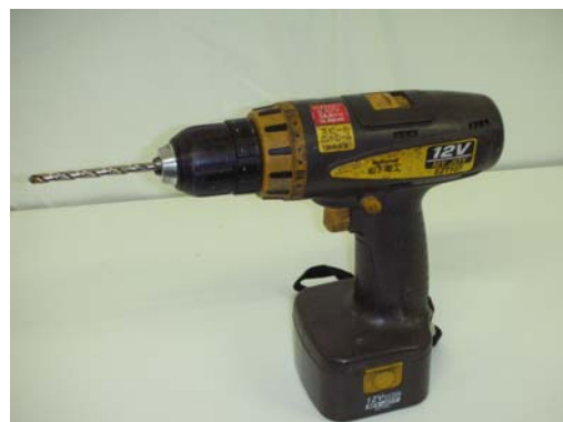
Photo 8 Process 3 Electric drill (Matsushita Electric Works MYJOY EZT107)
