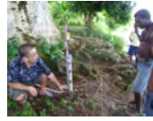
Water Level Gauge and Warning System operated by the community
