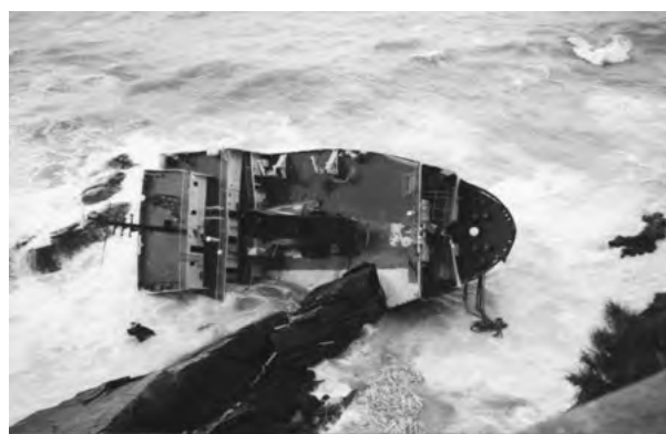
The stern section of the M/V LUJIN 2 impaling on a rock near the shore
