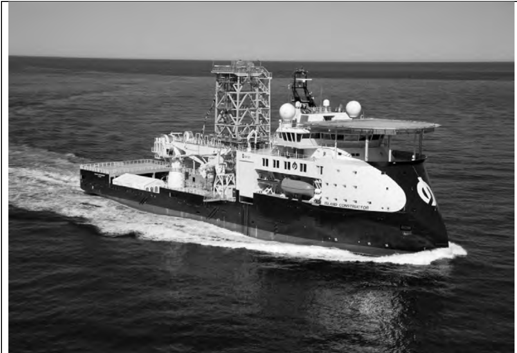
Riserless Well Intervention Vessel (RLWI) 写真提供 Islandoffshore (MOU Island Wellserver)
