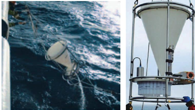
Figure 1-8 Sediment Trap Mooring System to sample falling solid particles in the ocean.
