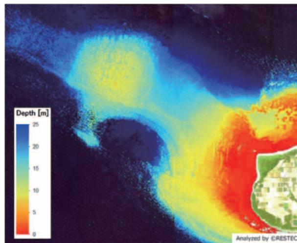
Figure 1-14 Coastal bathymetry derived from satellite Images
