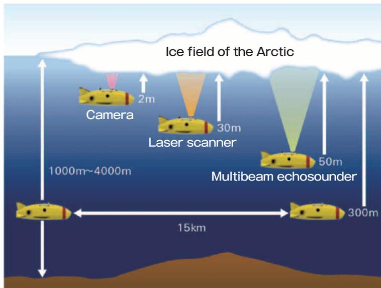
Figure 1-9 Schematic Illustration of comprehensive observation using multiple underwater observation drones.
