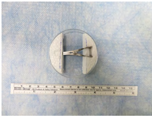
Figure 1 Graft preparation plate is modified by two foam blocks attached to a petri dish. A groove and hole were carved on the foam blocks to match the ends of a bulldog clamp.
