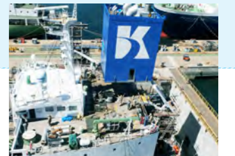
Photo:SANWA DOCK CO LTD Scrubber Chemical Tanker Retrofitting
