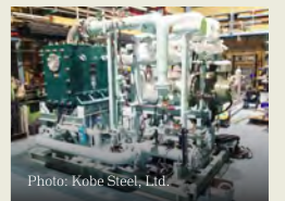
Photo: Kobe Steel, Ltd. Binary cycle power generation system for ships
