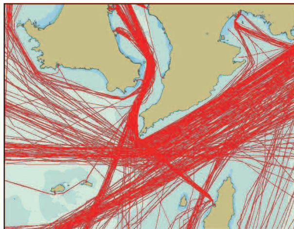
Figure 5-3 Example of how vessel movement is captured through the AIS (around the Osumi Peninsula) (Source : 10th Regional Coast Guard Headquarters)
