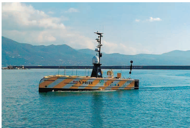
Figure 2-4 Autonomous seafloor mapping system developed by GEBCO-NF Alumni Team
