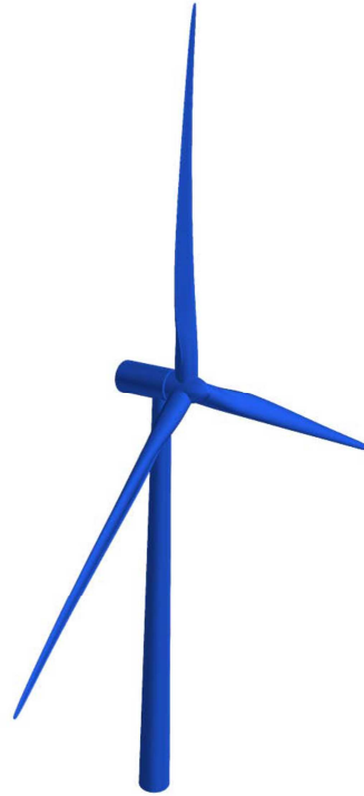
図 4.1 : DTU Reference Wind Turbine (出典: Christian Bak , “The DTU 10-MW Reference Wind Turbine” )
