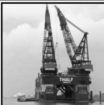
Siapem 7000 and Heerema Thialf Semi-Submersible Crane Vessels
