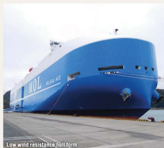
Low wind resistance hull form
