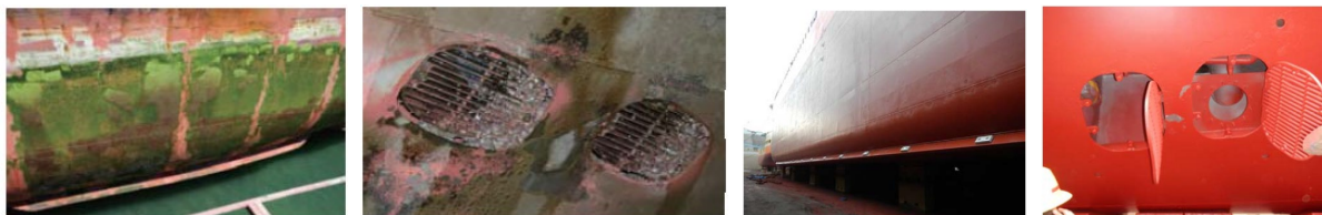
Biofouling on ship's surface before cleaning
