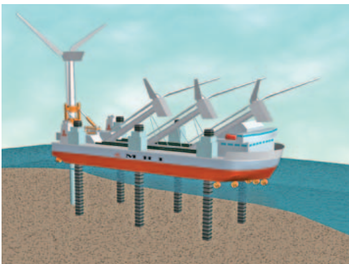
Developing ship designed for installation of offshore wind turbines (Example 1)
