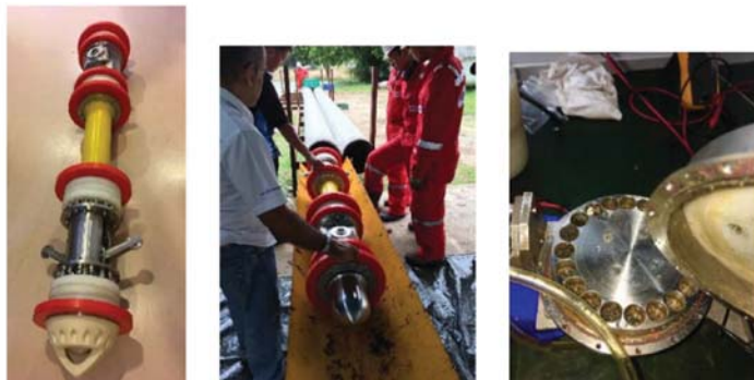
Figure 11—The specialized in-line pig equipped with sampling tool designed, developed and successfully tested in a company pipeline loop.(Left – Prototype Pig, Middle – Functional test, Right – Samples collecting section)
