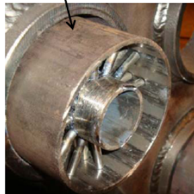
Basic Boiler Element configuration
