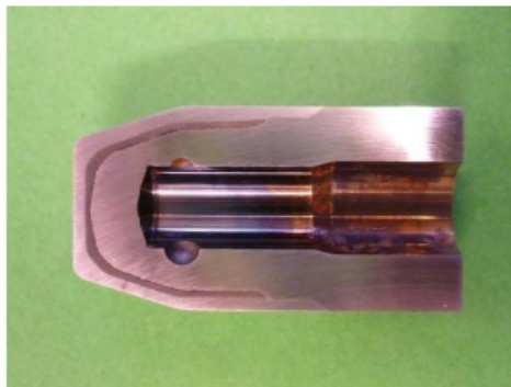
Sectioned prototype insulated nozzle.
