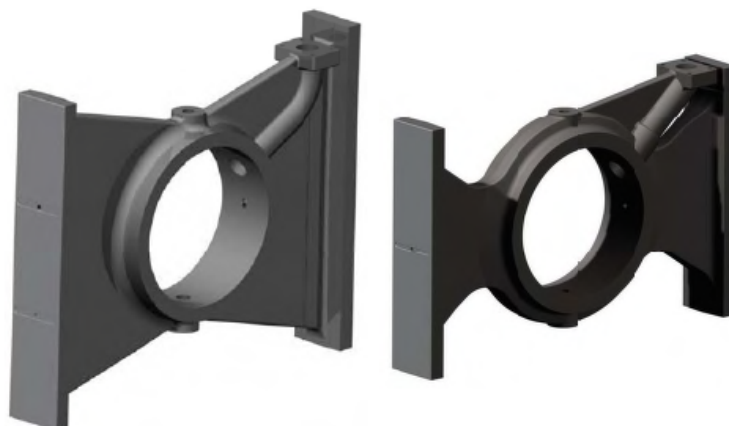
Standard Design of the K98ME-C Guide Shoe Power loss =18.3 kW/shoe
