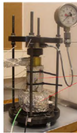
Test rig to determine heat transfer coefficients
