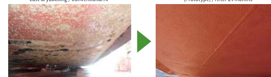
SEAFLO NEO M1 PLUS can reduce a risk of barnacle fouling in static condition and low activity operation.
