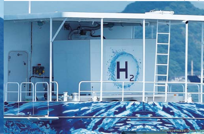
Movable hydrogen storage tank
