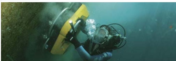
Diver performing underwater hull cleaning, Source: Hydrex
