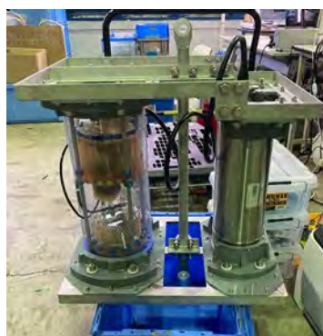
Observation equipment (eDNA Sampler) developed by JAMSTEC and attached to the mooring system.
