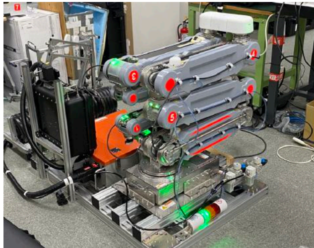
The arm with the downward configuration in its home location. The system can be very compact allowing the deployment in very narrow conditions.
