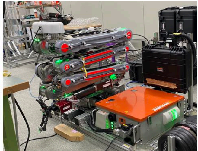
The arm with the downward configuration in its home location. The system can be very compact allowing the deployment in very narrow conditions.
