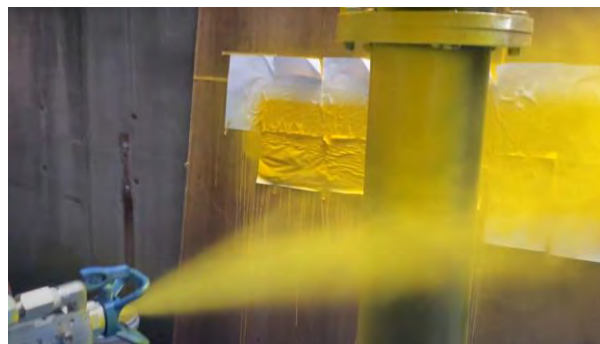
Pipe painting with adjusted settings (pressure: 1000 psi, distance 12in, robot speed 90%)
