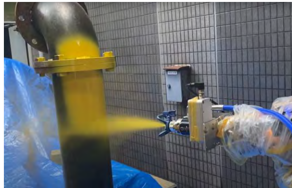
First attempt in pipe painting (pressure: 1000 psi, distance 12in, robot speed 60%)
