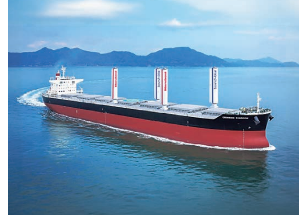
Project image for the panamax bulk carrier installed wind-assisted propulsion systems
