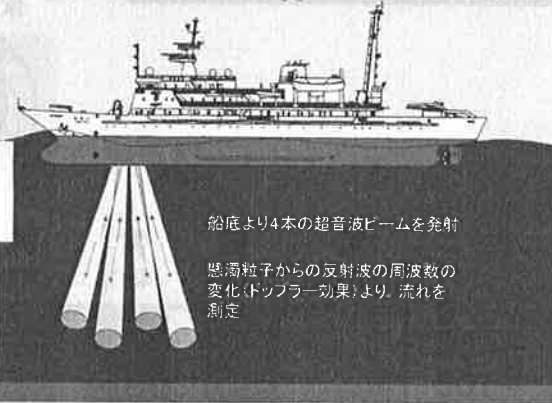
望星丸のAcoustic Doppler Current Profiler
